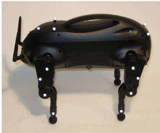
Figure 6: Robot Zero Configuration Position
