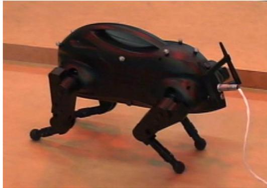
*Fig. 2:* The Little Dog quadruped robot
